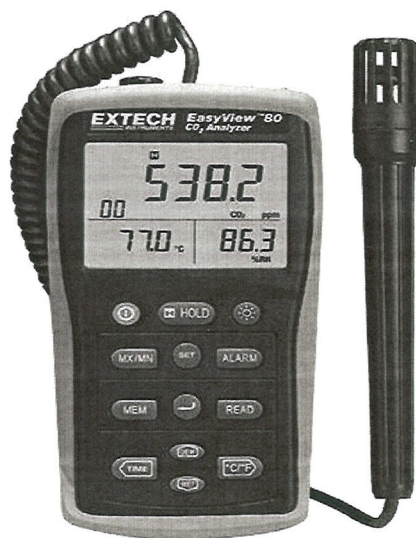
Figure 18. Indoor air quality meter
